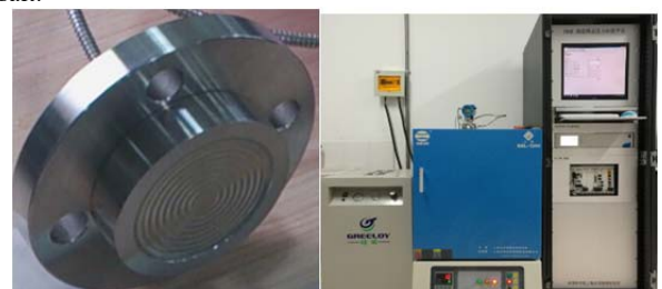
Fig.16 The filling NaK pressure transmitter and calibration bench
