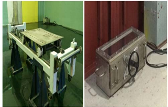
Fig.9 The round trip beam device and the irradiation box with different temperature and atmosphere
