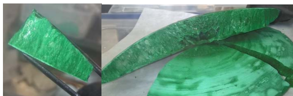
Fig.3 Photo of the fuel salts prepared by “one pot process”
