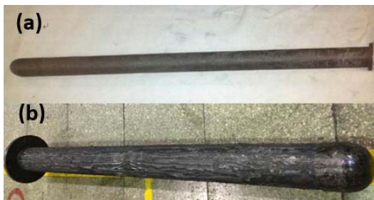
Fig.12 Prototype of control rod casing developed by hot isostatic pressing (a) and resin impregnation(b) process
