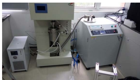
Fig.1 Test system for saturation vapor pressure of molten salt
