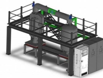
Fig.19 The high temperature ultrasonic flowmeter calibration platform
