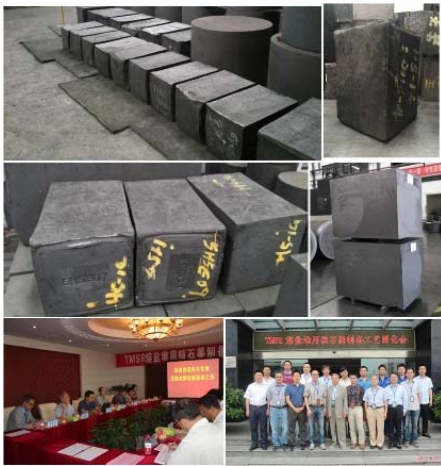
Fig.8 The witness of producing process of anti-molten salt infiltration of fine graphite material with size of 400×400×600 mm
