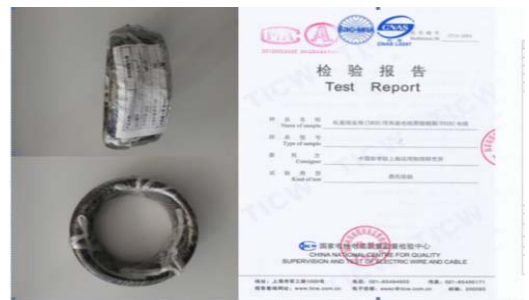
Fig.7 The high-temperature PEEK cable sample and the test report
