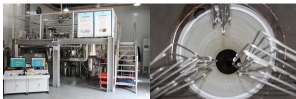
Fig.3 Picture of frozen-wall facility and image of the formed frozen wall
