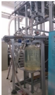
Fig.4 The fuel ball loading and unloading mechanism of TMSR-SF1
