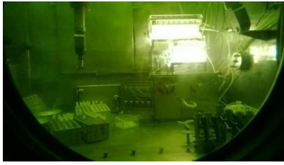
Fig.2 The “trace” bench experiment of uranium extraction process in “hot” cell
