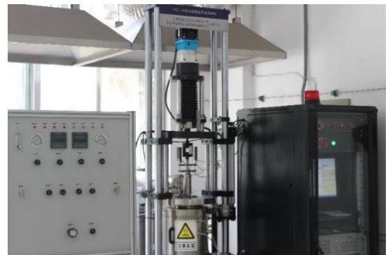
Fig.4 Molten salt environment in-situ materials tensile tester
