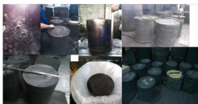
Fig.10 Anti-molten salt infiltration of fine graphite material \Phi 400 \times 400 mm process witness picture
