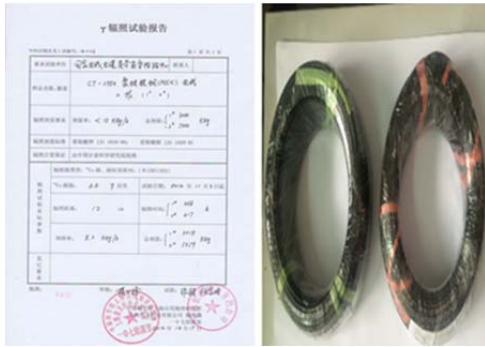
Fig.5 The PEEK high temperature nuclear power cable and the gamma-ray irradiation aging experiment
