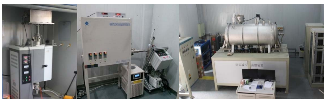
Fig.4 The distillation equipment of fluoride melt (Left: gram-scale vacuum thermogravimetric system; Middle: 100 gram-scale fully sealed distillation device; Right: kg-scale horizontal distillation facility)
