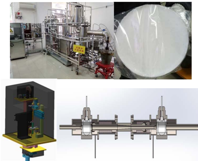
Fig.2 Pilot plant with a capacity of 5 kg FLiNaK per batch (up left), photograph of high quality FLiNaK (up right), 3 D models of of online sampler (down left) and transferring valve (down right)
