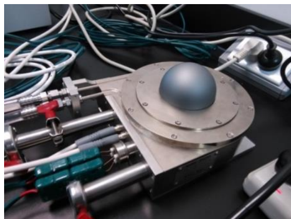
Fig.6 High temperature beryllium dome hotstage
