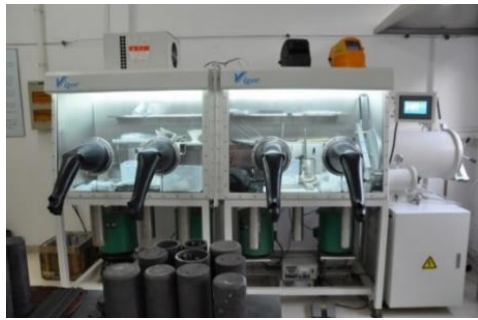
(a) FLiNaK corrosion experimental equipment
