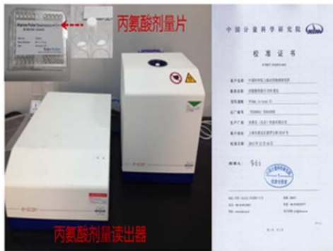
Fig.9 The ESR/alanine dosimeter dosage monitoring system and the certificate
