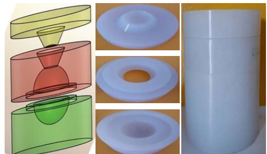
Fig.4 Design sketch and photos of Silicone Rubber mold
