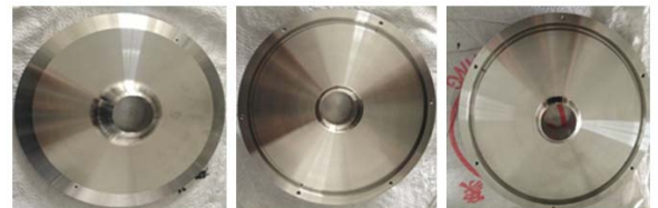
Fig.2 The figure of finished freeze flange
