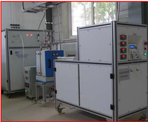
Fig.10 1 kW integrated SOEC evaluation platform.
