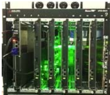
Fig.10 Prototype Reactor Protection System.
