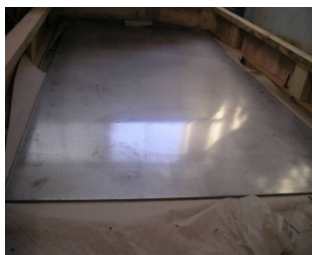
Fig.2 A rolled alloy GH3535 plat with size of 4 mm×950 mm×2000 mm.
