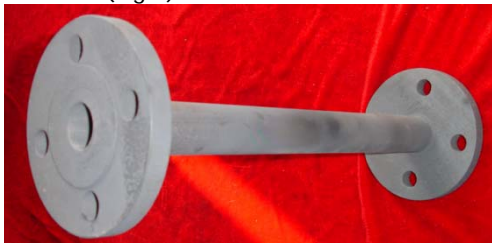
Fig.5 A C/C composite tube prepared (38 mm×440 mm).
