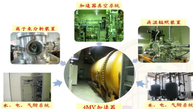
Fig.2 The 4 MV accelerator and ion beam irradiation chamber.
