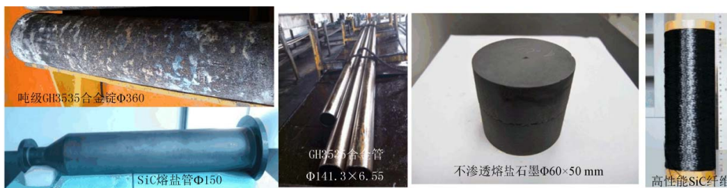
Fig.3 Molten salt reactor materials developed by TMSR center.
