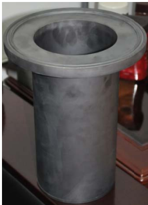
Fig.6 A pot made of sintered SiC.
