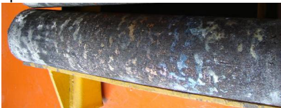
Fig.1 An alloy GH3535 ingot with diameter of 360 mm.
