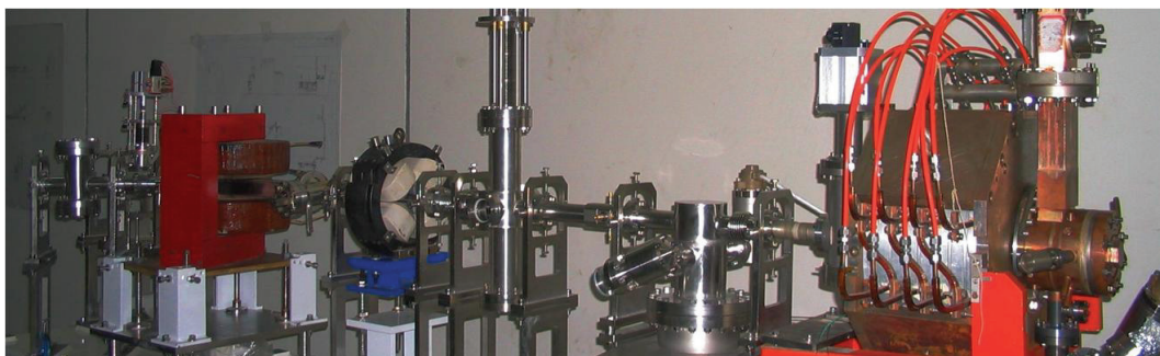
Fig.2 The beam line of the photocathode RF gun test bench.
